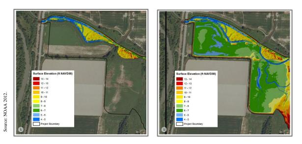
Figure 3-11. The Fisher Slough, WA Project boundary and the change in flood storage area before (left) and after (right) project completion.
