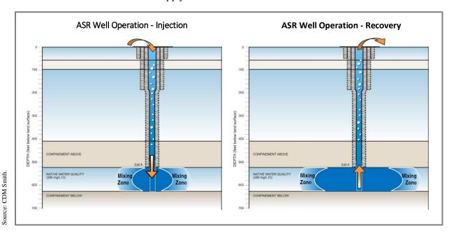
Figure 3-2. Typical ASR Well Operation
