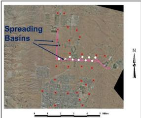
Figure 3-7. Injection Wells and Spreading Basins Interspersed in El Paso, Texas Water Supply Well field
