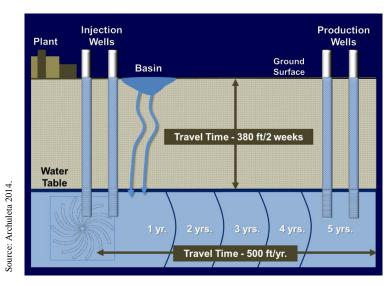
Figure 3-4. Typical ARAR System Operation
